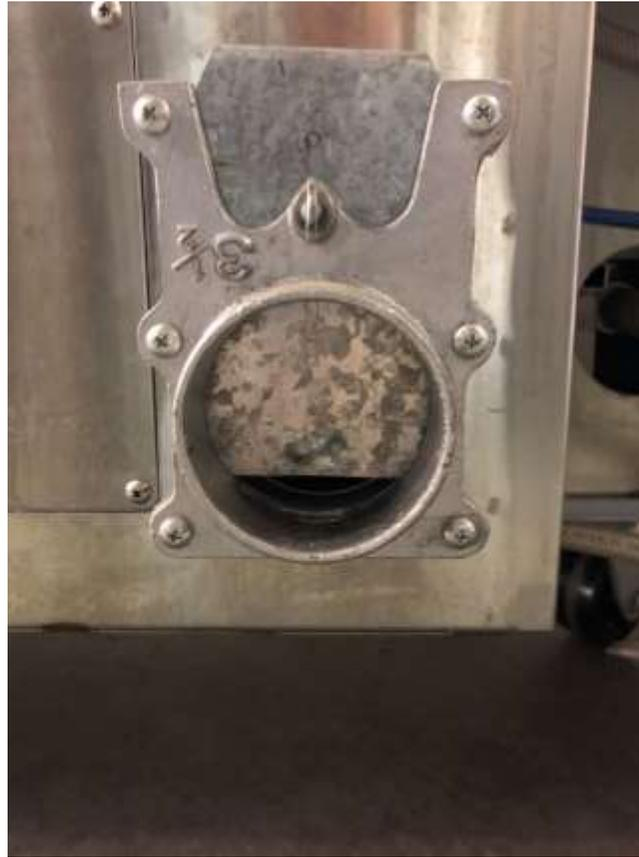
There is also an exhaust damper located on the rear of the console. This is to expel the humidity laden moist air. The dryer dries by moving a large volume of dry air over the items to be dried. The dryer is not an oven. An oven dryer would likely use temperatures in excess of 212° F that would likely boil off the water and may leave water mark residue.
