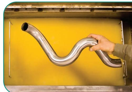
*The tube has been thoroughly cleaned inside and out in a hands-off process, saving precious and costly labor time.*
