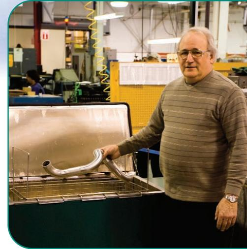
*Manufacturing Engineer Bud Greener loads a precision-bent tube into an Omegasonics ultrasonic cleaning system.*
