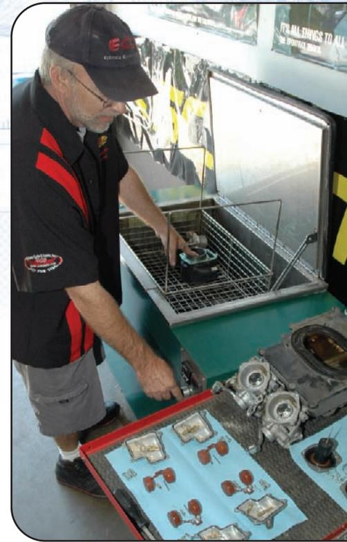
*The Omegasonics Pro Plus handles all types of motorsports engine components.*
